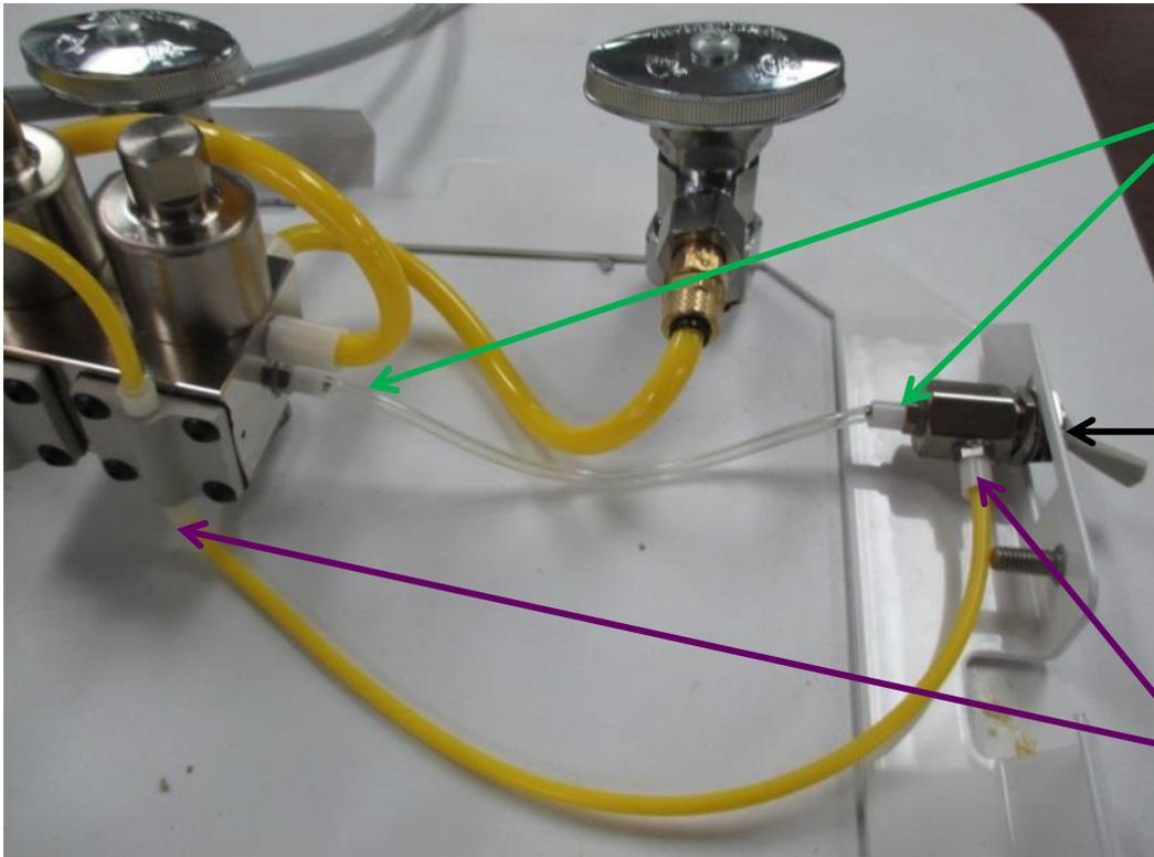
Connect constant air to the barb farthest away from the toggle (input) on the master on/off valve.
